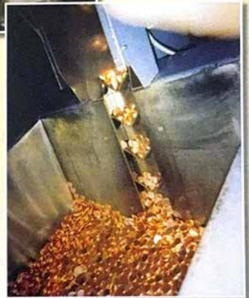
Figure 2: Cent planchets being fed into the feeder mechanism prior to striking.
