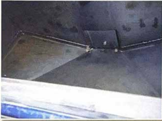
Figure 7: This picture of a tote bin clearly shows a few leftover blank planchets trapped at the bottom near the "trap door." If this tote bin were used in the production of coins of a different denomination without being thoroughly inspected by Mint personnel, the leftover planchets could be struck into wrong planchet errors.
