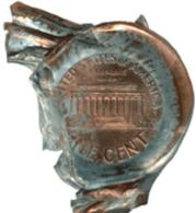
Donded coins occur when the feeder system, which supplies blank planchets to the coin press, malfunctions and jams. When this occurs, a struck coin is not properly ejected and another planchet is fed into the collar and is struck. This struck coin will land on top of the previously unejected strike. These coins will then crush and bond together. This may occur many times as more coins bond.
