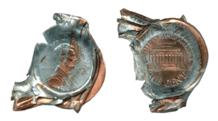
Bonded coins are created when the feeder system, which supplies blank planchets to the coin press, malfunctions and jams. When this occurs, a struck coin is not properly ejected and another planchet is fed into the collar and is struck. This struck coin will land on top of the previously unejected strike. These coins will then crush and bond together. This may happen multiple times as more coins bond.
