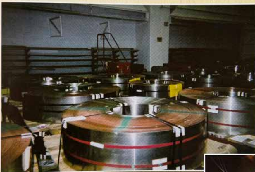
Figure 1: These rolled strips will eventually be punched into blank planchets for Quarters.
