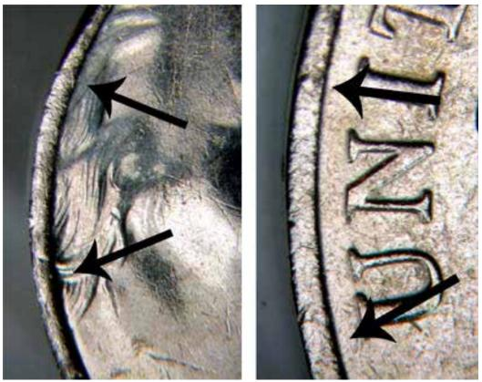
**Photo 5:** The broad and flat rims area opposing the clip, where the planchet was not upset. Obverse is at left, and reverse at right.
