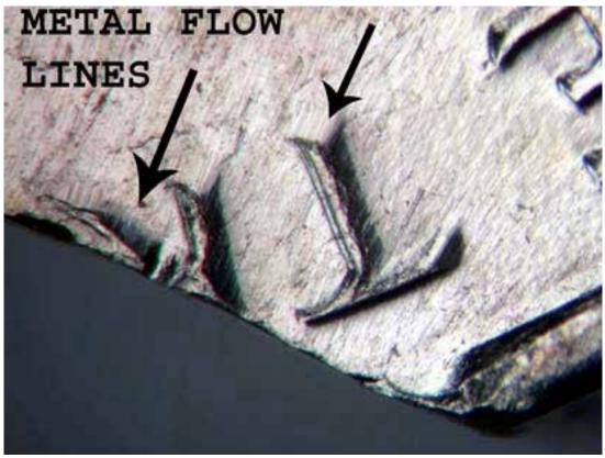
Photo 7: Another close-up of obverse clipped edge, also showing metal flow.
