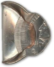
A fold-over coin is one of the most dramatic types of errors. It occurs when the blank is standing vertically between the dies. During the strike, the force is so great that it bends and folds the blank. These fold-overs can be on-center or off-center, and come in many different shapes. There are a few fold-overs with multiple errors, either with an additional strike or fold-over. Denominations above quarters are very scarce.
