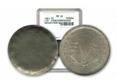
A counterbrockage error involves a cap die and a previously struck coin. When a cap die strikes a previously struck coin, the obverse design from that struck coin will be impressed into the cap. The result will be a design where the cap face will be an incuse brockage. When a new blank is struck by this cap die with an incuse brockage image, the obverse will have a raised and spread image from that incuse design of the cap. This brockage impression is known as a counterbrockage.
