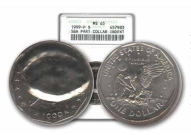
A n indent error occurs when two blanks are fed inadvertently into the same collar, with one blank partly overlaying on top of the other. When the hammer die strikes this combination, the upper blank will be forced into the lower blank, creating a depression which is shaped similar to the upper blank. A scarce type of indent occurs when a blank intended for one denomination lands on top of a blank from a different denomination.
