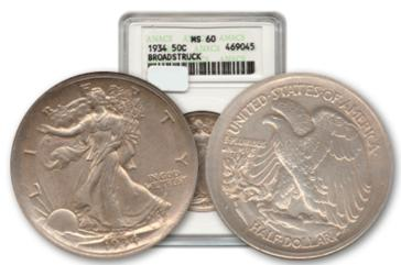
A broadstruck error occurs when a coin is struck without the collar to form the rim and edge that is part of the shape of the coin. Coins can be broadstruck on either type one or type two planchets. When a coin is broadstruck the blank being fed into the collar will spread and distort outward as it is being struck because the collar isn't in the correct position to retain it.
