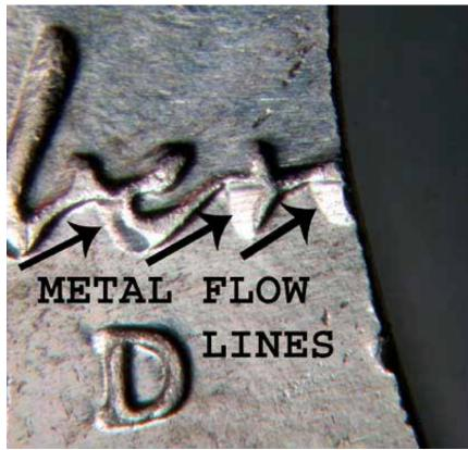
**Photo 6:** A close up of obverse clipped edge, showing distinctive directional metal.
