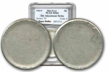
Die adjustment strikes are also known as die trials. This error occurs when a coin is struck from the press with very little pressure. When the press is being set up and adjusted, extremely weak strikes occur as the strike pressure reaches its optimum level. These die trials are destroyed after being struck and are rarely found in circulation.
