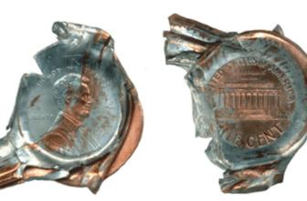
**B** onded coins occur when the feeder system, which supplies blank planchets to the coin press, malfunctions and jams. When this occurs, a struck coin is not properly ejected and another planchet is fed into the collar and is struck. This struck coin will land on top of the previously unejected strike. These coins will then crush and bond together. This may occur many times as more coins bond.
