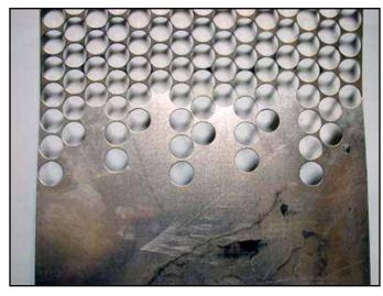
Photo 3: A strip from which planchet blanks are cut.
