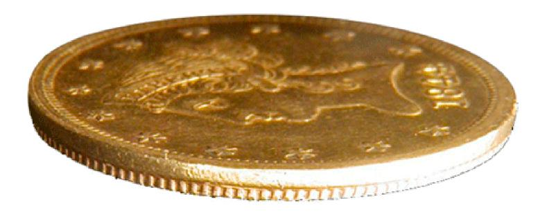
Partial collar strikes occur when there is a malfunction of the striking press. This causes the collar to be in an incorrect position. The lower die (usually the reverse die) is recessed in the collar. This allows the coin which is going to be struck to have a formed rim. After a coin is struck the lower die raises upwards, pushing the struck coin out of the collar and ejecting it.
