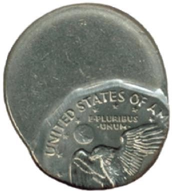
Off-center coins are one of the most common and best known types of errors. This happens when a blank which is supposed to be fed into the press, lands in the collar improperly. When this occurs only part of the blank is between the upper and lower dies. When the dies strike the blank, only that part will be struck with a design.
