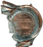
B onded coins occur when the feeder system, which supplies blank planchets to the coin press, malfunctions and jams. When this occurs, a struck coin is not properly ejected and another planchet is fed into the collar and is struck. This struck coin will land on top of the previously unejected strike. These coins will then crush and bond together. This may occur many times as more coins bond.
